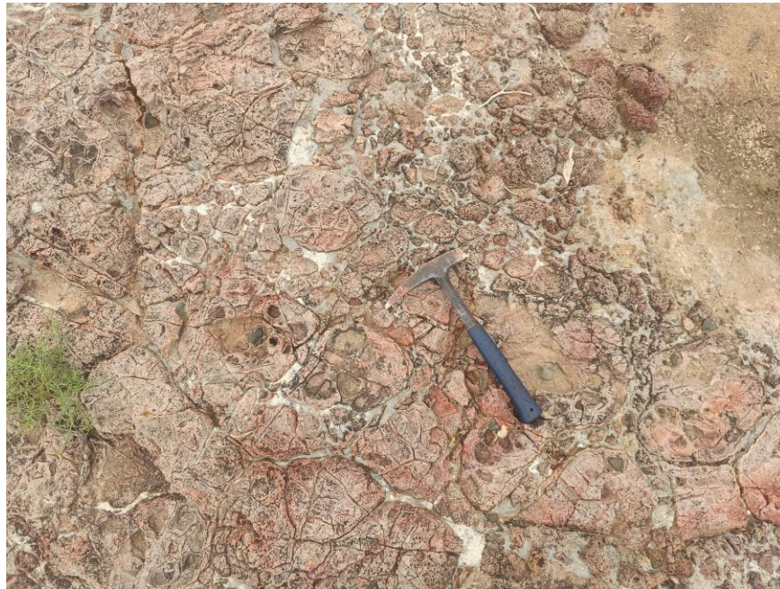
Photograph No. 7.3: Exposure of pisolitic-oolitic lateritic bauxite characterized by rounded ferruginous concretions embedded in a clayey lateritic matrix.
