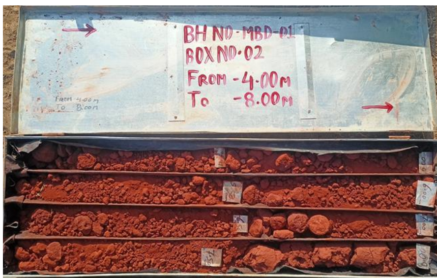
Photograph No.13.3: Drilled core by dry drilling
