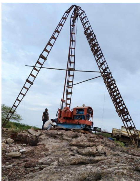
Photograph No.13.1: RD60 drill Rig used for drilling operations
