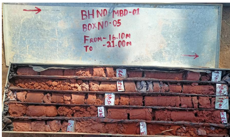
Photograph No.13.4: Drilled core by dry drilling
