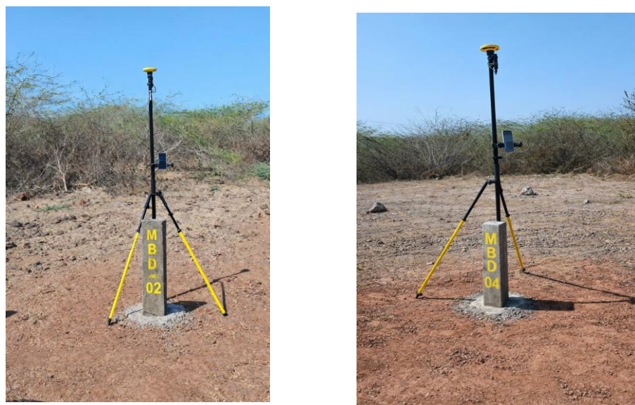
Photograph No.13.2: Pillars constructed on boreholes drilled in Dhrang block by MECL.
