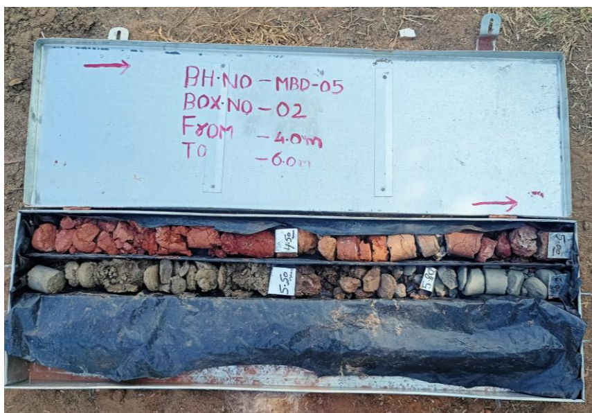
Photograph No.7.9: Core Photograph of MBD-05 showing Lithomargic clay intercepted between 4.71m to 5.50m
