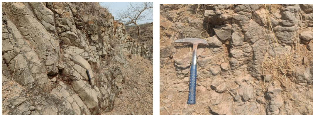
Photographs No. 7.11A & B: Porphyritic Basalt and Amygdaloidal Basalt
