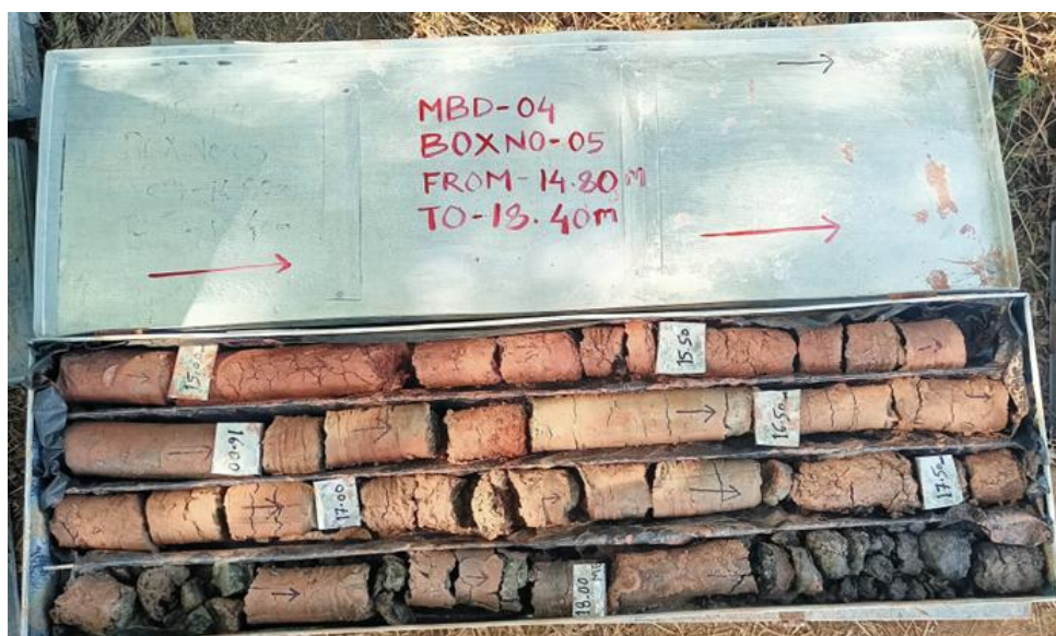
Photograph No.7.8: Core Photograph of MBD-04 showing Bauxitic Clay intercepted between 15.00 to 17.00m
