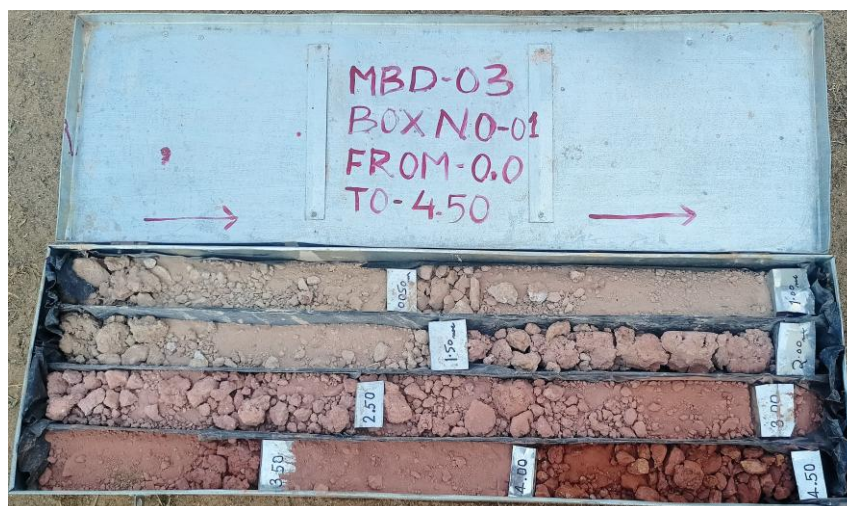
Photograph No.7.7: Core Photograph of MBD-03 showing Clayey Bauxite intercepted between 0 to 4.00m
